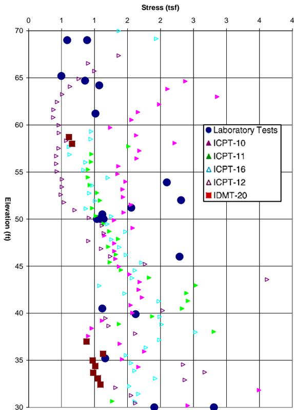
Figure 2a. IDMT-17 Undrained Shear Strength
