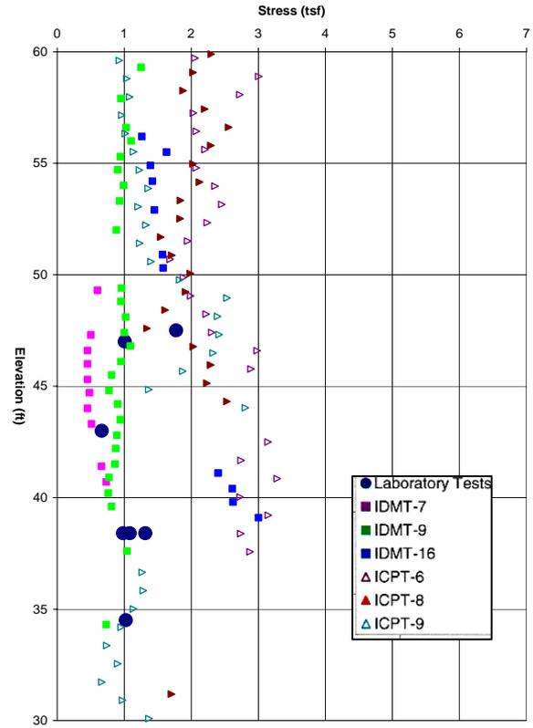
Figure 2c. IDMT-7, 9 & 16 - Undrained Shear Strength
